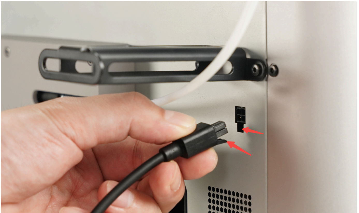
Bambu Bus Cable 4 pin ( Correct orientation)
