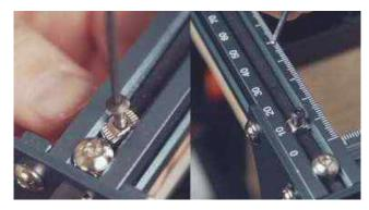
When mounting the limit switch, place the cut or printed spacer underneath the limit switch board, and oriented it such that the "arm" of the limit switch faces the head of the laser.
