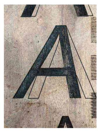
If your output looks like this, you likely have your motor pulse step polarity set incorrectly. On Ruida controllers, there's a setting called 'PWM Rising Edge Valid' that you can change for each axis that tells the controller whether the rising edge or falling edge of a step pulse is what the motor driver is looking for. Toggling this may fix skewed engraving.
