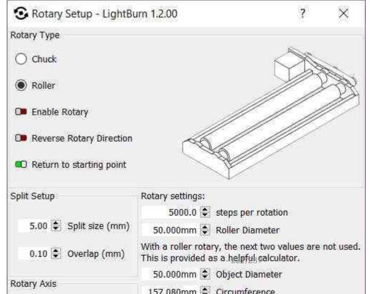
To use the rotary with your marking laser, you first need to set up the rotary parameters.
