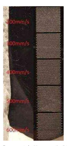
To compensate for this, measure the distance between the ends of the lines at each speed, and enter the speed and distance values into the scanning offset adjustment table. LightBurn will use this information to compute the correct adjustments for other speeds as well. A minimum of two measurements are needed for it to work. **Note** you will need enter *half* the measured value - The software moves each line by the amount you specify, so each pair of lines only needs to move half the distance.
