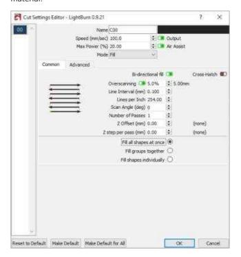
Run this rectangle at multiple speeds, like 100mm/sec, 200mm/sec, 300mm/sec, and so on. Depending on your hardware you may not even need to use these settings, however here is example output from a machine that does:
