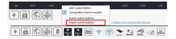
For Lightburn, it will prompt a 'New Device Wizard' or click "Devices" in the laser control module to import the engraver. Click 'Import', select the Nano Duo.lbdev file, and click OK to add the Nano Duo configuration to LightBurn. The macro commands will be successfully added in the Console window and Nano Duo device
