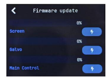
Note: When there is no new firmware in the SD card or the new firmware is not in the root directory of the SD card, the interface will display "Retrieval failed".
