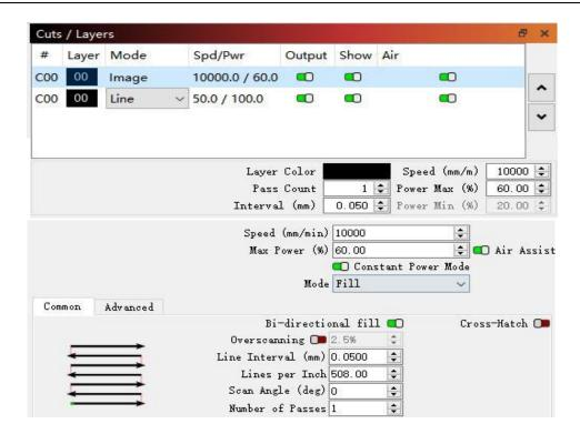
At high speed, if it is fill mode, the engraving effect is not good, you can change the Line interval to 0.025mm.
